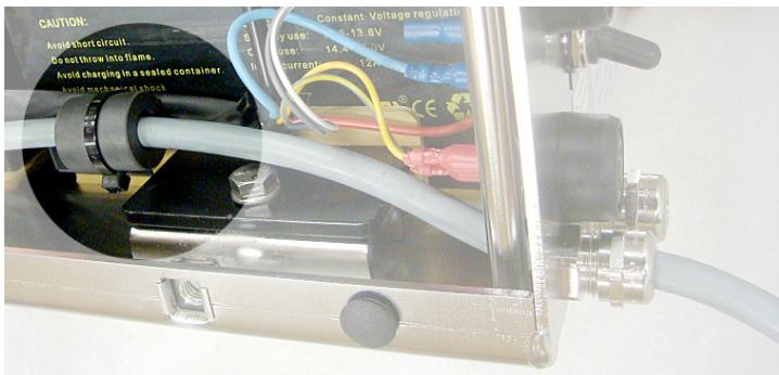
**IMPORTANT:** P-LIGHT® holds type approval to ECE No. 10. For this to be valid, the incoming cable connected to terminals 3-7 must be fitted through the installed ferrite core, as illustrated.
